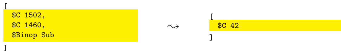
Figure 3.5: Reduction of a subtraction instruction (yellow) without any surrounding context.
